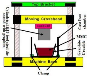
**Fig. 2**: Schematic diagram of squeeze casting process on UTM
