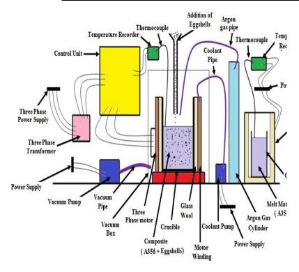
Fig. 1: Experimental Set-up of Electromagnetic Stir Casting Process
